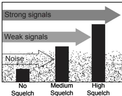
While listening to a channel, adjust the **SQUELCH** knob until the noise is filtered and you can hear only the transmission. If you switch to a channel with a lot of noise or a weak transmission, you may need to readjust the squelch level again.
