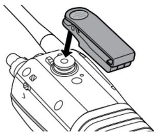
1. Rotate the belt clip so that the finger indentation is towards the top of the radio.
