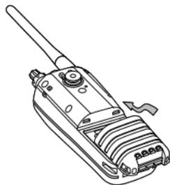
2. Lower the battery until it rests flat in the compartment.
