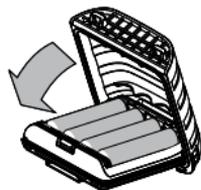
**NOTE:** Each time you open the battery case, check the rubber seal. Make sure the seal is seated in the groove and there is no dirt or debris on it. If the rubber seal looks worn or damaged, contact customer service to order a replacement (see the back cover page for contact information).
